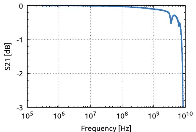
Figure 2: Frequency response (insertion loss) S21 (S12) versus frequency
