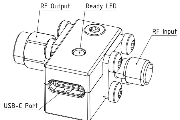
Figure 8: TVS-5VRR overload protection with 50 Ω SMA (female) input and SMA (male) output. The USB-C port is used for power supply. The green LED indicates active power supply required for proper operation of the protection device.
