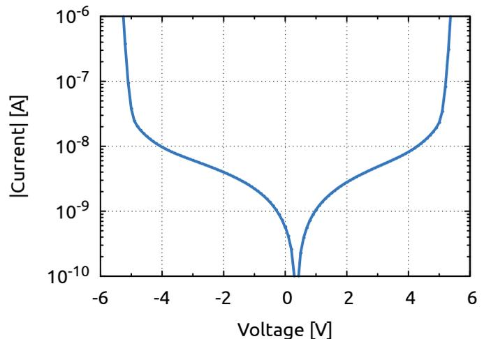
Figure 1: DC characteristic. The current is plotted as absolute value for negative input voltage. Measured with Keithley 2400 SMU in 4-wire mode and sweep start from zero for both polarities.
