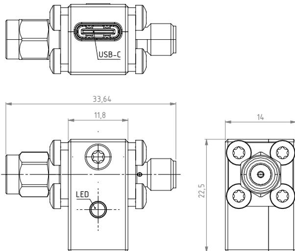
Figure 9: TVS-5VRR enclosure dimensions in [mm]
