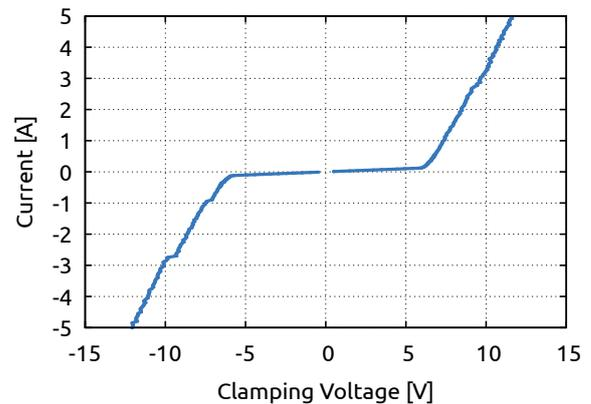
Figure 6: Clamping characteristic at 50 Ω, 100 ns pulse width, 100 ps rise time, 70 ns to 90 ns averaging window
