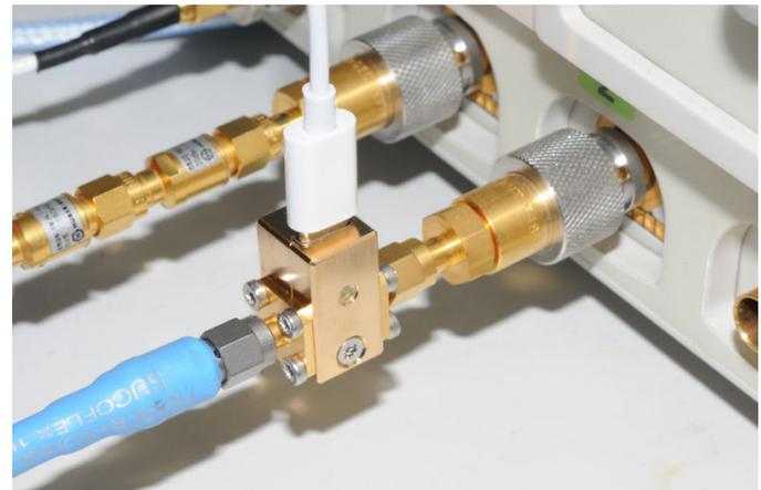
Figure 10: Application of the TVS-5VRR overload protection device, connected directly to the oscilloscope RF input. The USB-C port of the TVS-5VRR must be connected to any free USB port of the oscilloscope.
