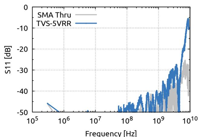
Figure 3: S11 (S22) versus frequency. For reference a SMA (female/female) thru is also shown.
