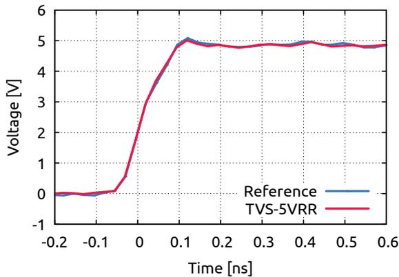
Figure 4: Step response at 100 ps rise time measured with 12 GHz bandwidth at 40 GS/s sampling rate
