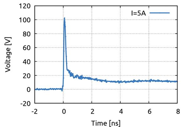
Figure 7: Overshoot and clamping characteristic at 5 A or 250 V overload into 50 Ω at 100 ps rise time and 100 ns pulse width
