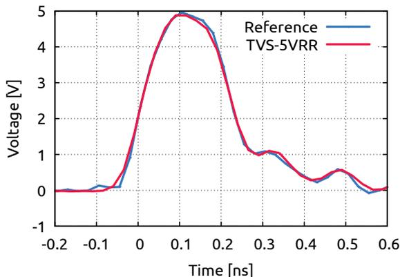
Figure 5: VF-TLP pulse transfer characteristic at 100 ps rise time and 230 ps pulse width measured with 12 GHz bandwidth at 40 GS/s sampling rate
