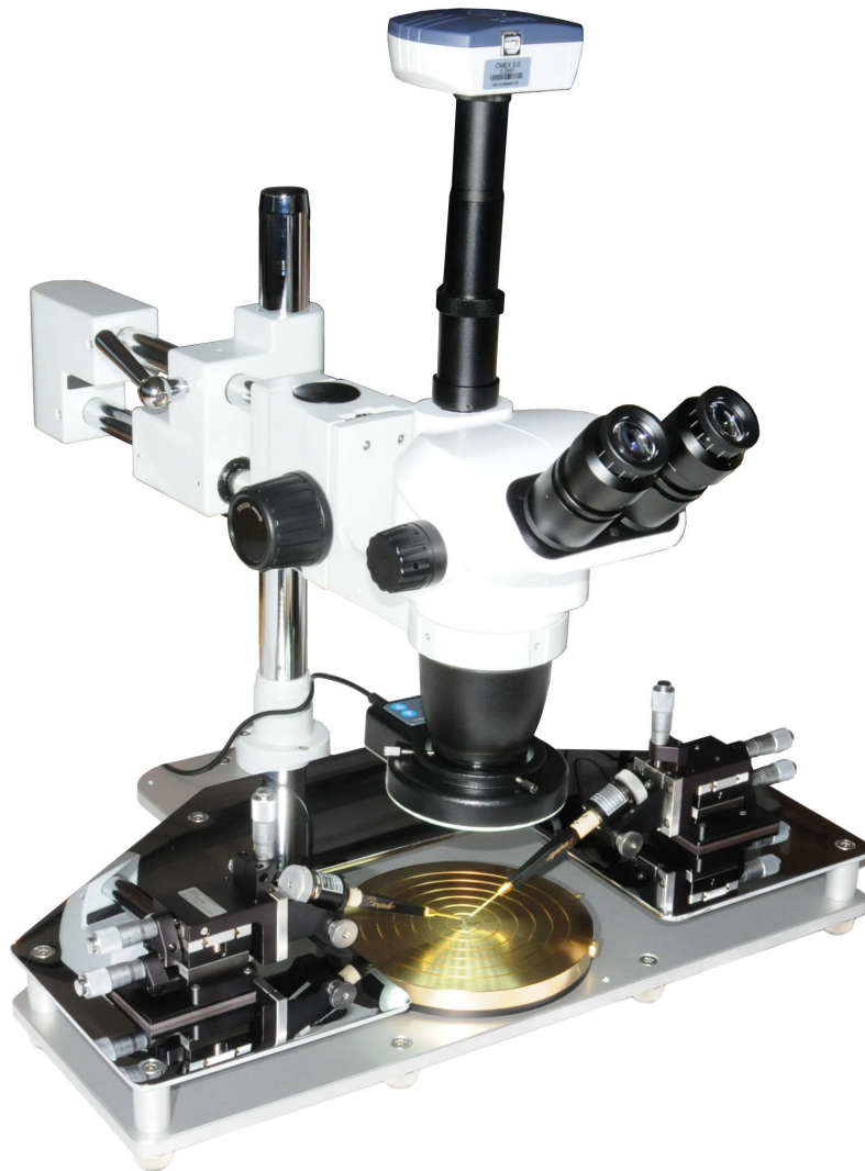
Figure 4: PS-5026B portable wafer probe station with 5 MP USB video camera. Optional: precision Picoprobe ® micropositioner Kit PHD-3001A, two micropositioner from Quater ® model XYZ500TIM.
