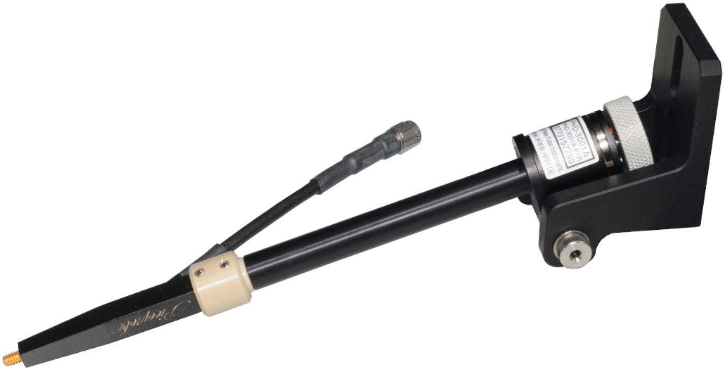
Figure 10: Photograph of shaft extension (PPM10_H7)
