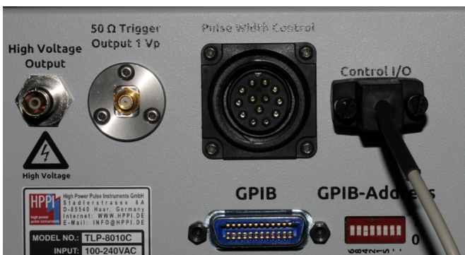
Figure 8: Interlock interconnection cable connected to the Control I/O port
