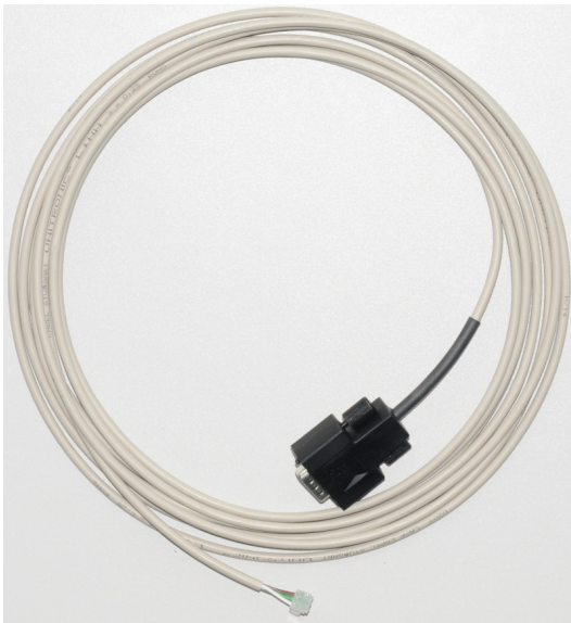
Figure 6: Interlock interconnection cable
