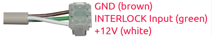
Figure 9: Pin diagram of the 3-pin 2.54 mm header on the interlock interconnection cable
