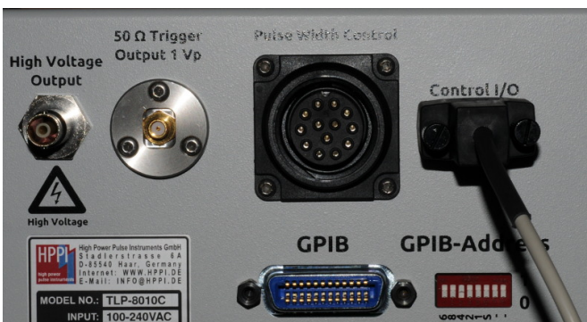
Figure 8: Interlock interlock connection cable connected to the Control I/O port
