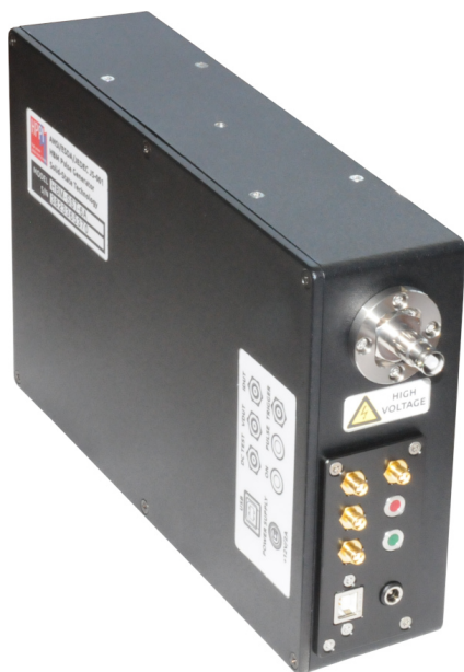
Figure 2: HBM pulse generator HBM-SST-6A ( \pm 6 kV)
