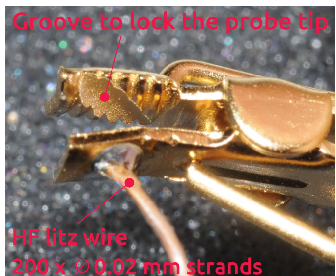
Figure 4: Unique groove locking in the brackets of left- and right sided clamp for solid electrical contact, precise locking and easy use. Gold coating for high contact reliability. High conductivity and low inductance copper HF litz wire with 200 x Ø 0.02 mm strands.
