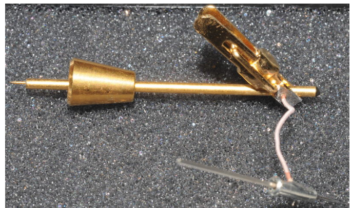
Figure 8: Left-sided locked probe tip
