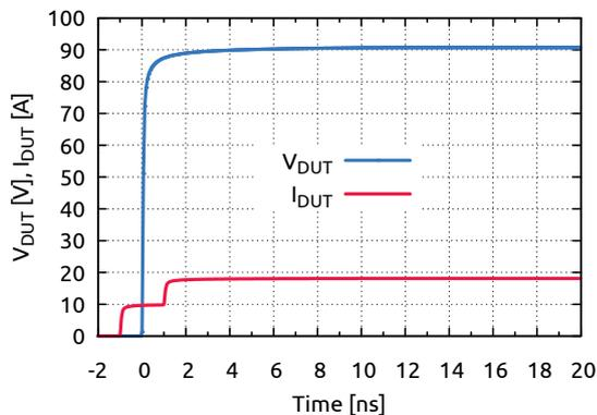
Figure 5: Simulated DUT waveforms with  $L = 0.2$  m condition
