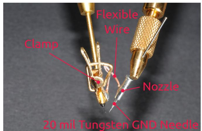
Figure 11: Ground fixture GF-A / 15 mm assembly: clamp, flexible wire and nozzle including 20 mil (0.508 mm) tungsten GND needle
