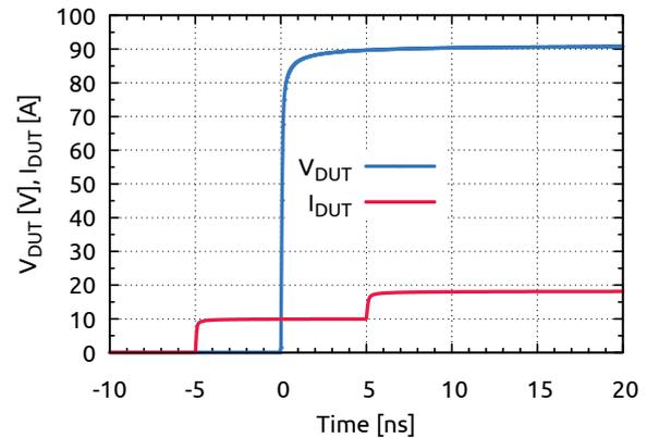
Figure 6: Simulated DUT waveforms with  $L = 1$  m condition
