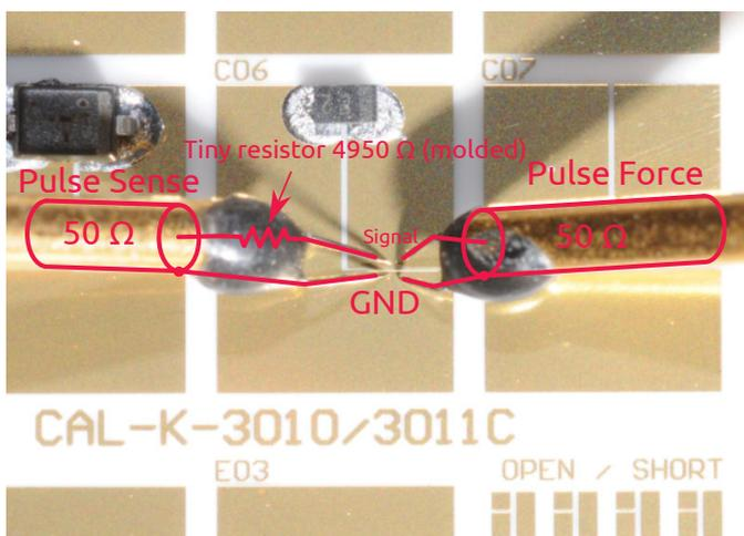
Figure 9: Fixed pitch picoprobes. Probing a reference device on the TLP calibration substrate. Detail view of Fig. 8 including equivalent circuit of the probe tips.
