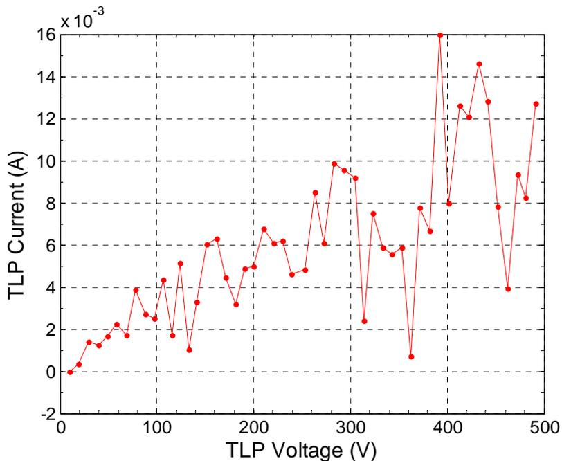
Figure 18: I-V curve measured over an open with a 2.5 ns wide pulse with 100 ps rise time. The data is averaged from 1 to 2.2 ns. **Note: y-axis shows milliamperes.**
