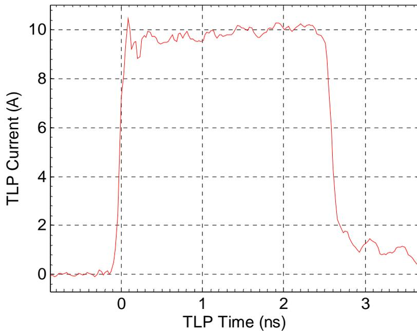
Figure 5: Measured transient current during a 2.5 ns, 100 ps rise time, 10 A pulse into a short (Fig. 2).
