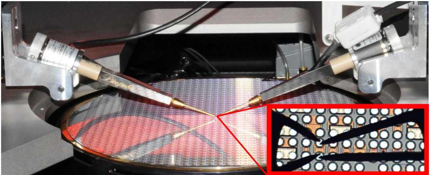
Figure 10: Kelvin setup with Picoprobe model-10. The right probe has an integrated 2.5 k resistor to sense the voltage with minimal load.
