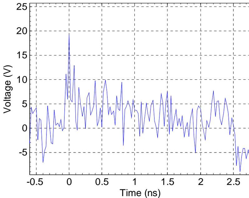
Figure 16: Transient voltage curve during a 2.5 ns, 100 ps rise time, 10 A pulse into the short. 10 pulses were averaged to decrease noise. In this plot the  $0.25\ \Omega$  series resistance has not been subtracted.
