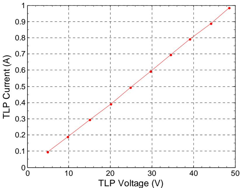
Figure 19: I-V curve measured over a 50 Ω load with a 2.5 ns wide pulse with 100 ps rise time. The data is averaged from 1 to 2.2 ns.
