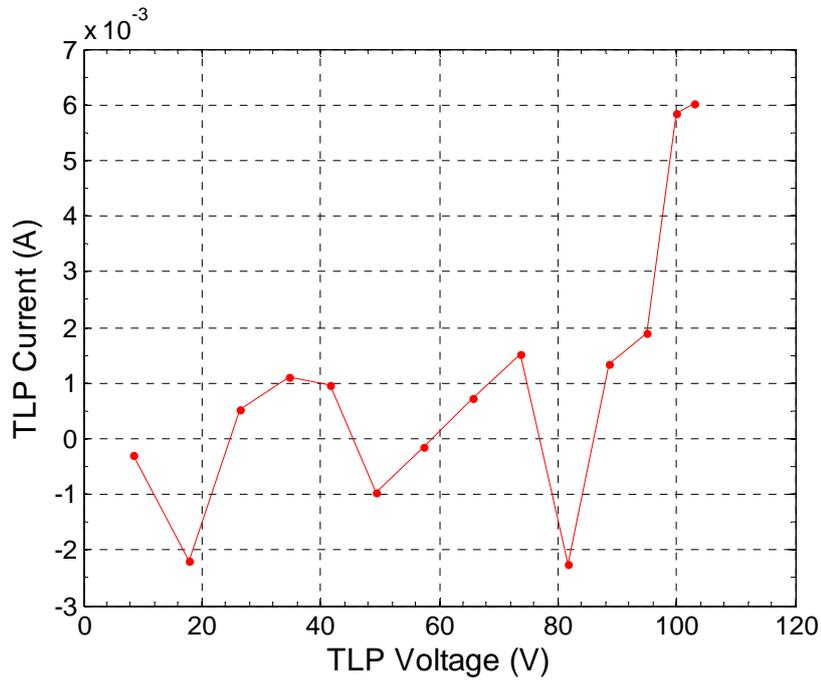
Figure 6: I-V curve measured over an open circuit with a 2.5 ns wide pulse with 100 ps rise time. The data is averaged from 1 to 2.2 ns. **Note: y-axis shows milliamperes.**
