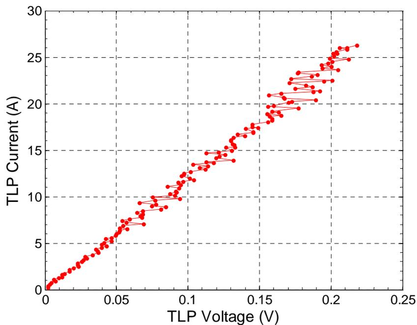
Figure 3: I-V curve measured over a short with a 2.5 ns wide pulse with 100 ps rise time. The data is averaged from 1 to 2.2 ns. The low series resistance of approx.  $8\ \text{m}\Omega$  shows the advantage of the Kelvin method.
