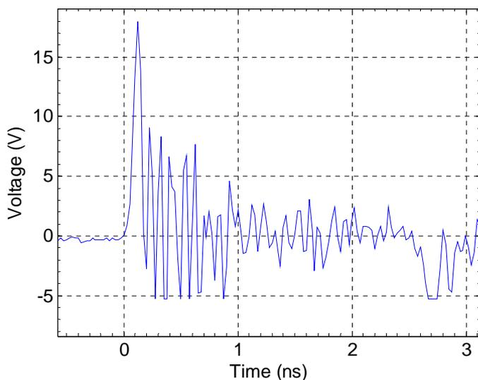
Figure 12: Transient voltage during a 2.5 ns, 100 ps rise time, 10 A pulse into a short. The ringing is caused by inductive coupling between the force and sense probes. **Note:** The scope bandwidth is 12 GHz and the noise is in the 10 GHz range. Since the bandwidth of the sense probe is limited to 5 GHz it would be favorable to apply a digital filter or use an analog low-pass filter.
