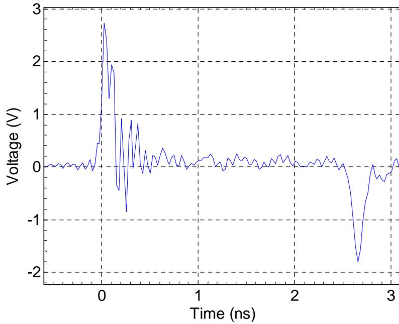
Figure 4: Measured Transient voltage during a 2.5 ns, 100 ps rise time, 10 A pulse into a short (Fig. 2). The overshoot is caused by the inductance of the short circuit plus inductive coupling between the force and sense probes.
