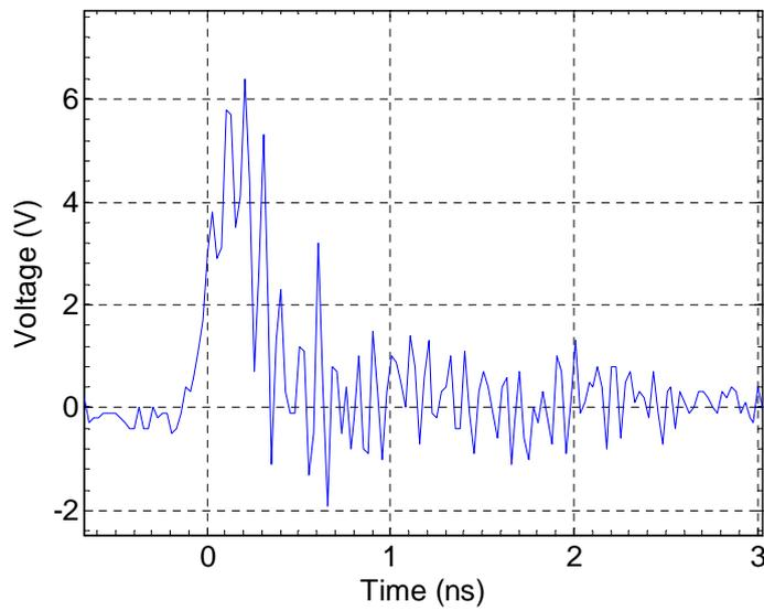
Figure 13: Transient voltage during a 5 ns, 300 ps rise time, 10 A pulse into a short. In comparison to fig. 12 the ringing is lower due to the slower pulse flank.
