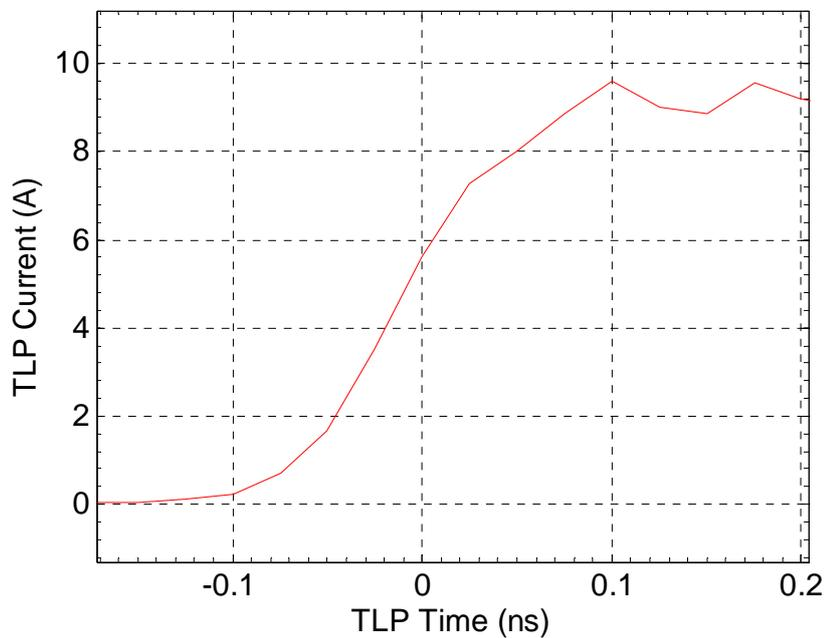
(b) Current waveform: detail view of rise time.
