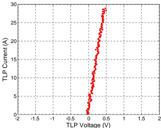
Figure 11: I-V curve measured over a short with a 2.5 ns wide pulse with 100 ps rise time. The data is averaged from 1 to 2.2 ns. Since the measurement is measured with a Kelvin setup there is no need of subtracting series resistance. The Ron of about 17 mΩ is rather the resistance of the metal itself.
