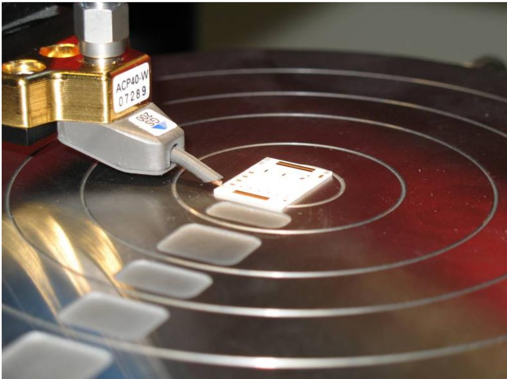
Figure 14: The measurement was performed on a calibration substrate. The inset figure shows a short circuit contacted with a probe with 200  $\mu\text{m}$  pitch.
