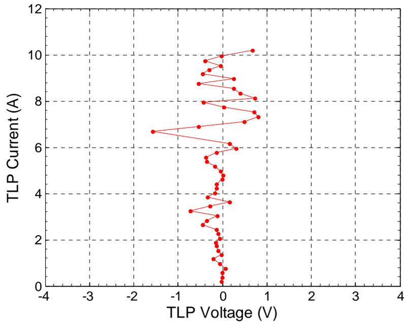
Figure 15: I-V curve measured over a short with a 2.5 ns wide pulse with 100 ps rise time. The data is averaged from 1 to 2.2 ns. The noise is related to the inaccuracy of the oscilloscope when two large amplitudes are subtracted. A parasitic contact resistance of  $0.25\ \Omega$  has been subtracted from the voltage.
