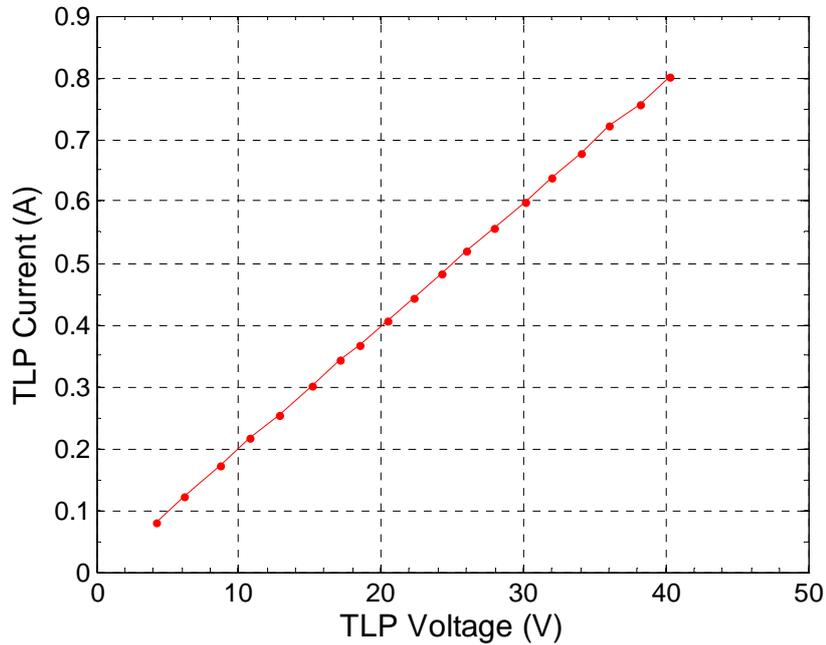
Figure 8: I-V curve measured over a 50 Ω load with a 2.5 ns wide pulse with 100 ps rise time. The data is averaged from 1 to 2.2 ns.
