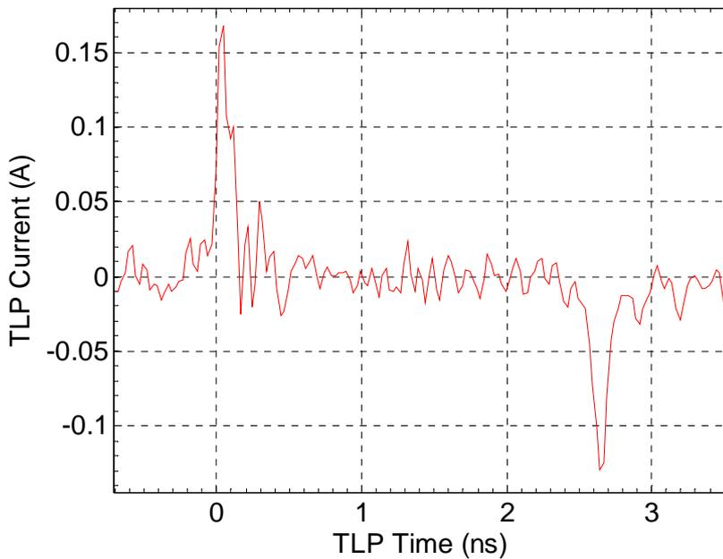
Figure 7: Measured transient current during a 2.5 ns, 100 ps rise time, 100 V pulse into an open circuit on a calibration substrate. A small capacitive current flows during the first 100 ps.
