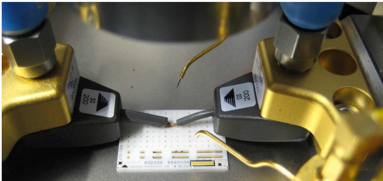
Figure 1: Kelvin setup with Cascade ACP-40 probes. The left probe has an integrated 1k resistor for direct voltage sense at the device pads.
