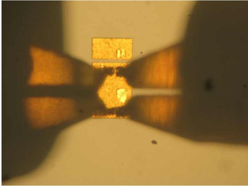
Figure 2: Microscope image of ACP-40 probe tips contacting a short circuit consisting of a massive copper area on the calibration substrate. The probe pitch is  $200\ \mu\text{m}$ .
