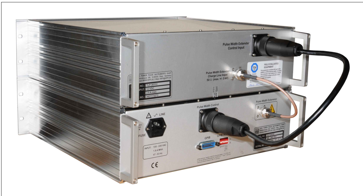
Figure 17: TLP-3010C/3011C rear panel electrical connections
